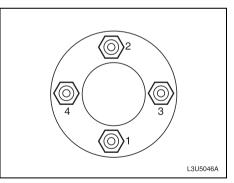
12)Tighten the wheel nuts firmly in a crisscross sequence as shown.
